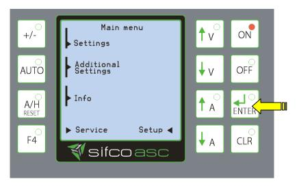
Select the desired menu point by pressing the corresponding key.
