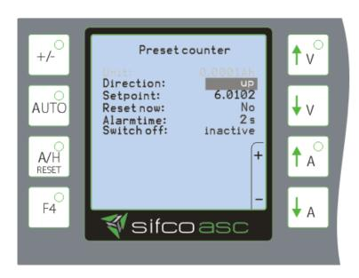
Select the desired item of the menu point "preset counter" by using the arrow keys.
