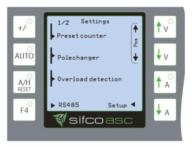
Select the desired sub item of the menu point by pressing the corresponding key.
